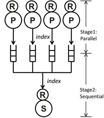
Figure 2: Pipeline generated for K-means by CGPA.
