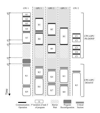
Figure 3: Flexible Execution: Run-time system adapts program configuration including task-to-core mapping to suit execution environment
